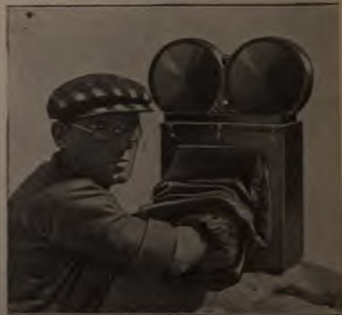
A Compact Dark Room for Motion-Picture Camera Operators: Inside the Wooden Box Are Bottles Containing Developing and Fixing Solutions
